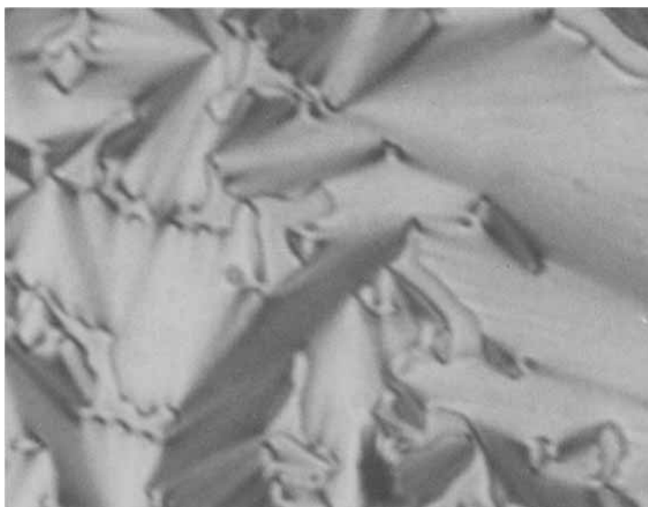
Fig.8 We present some typical textures for the DOBBA compound in the nematic phase (a) and of the complexes DOBBA-Cu(b) and HOBBA-Cu(c) in the smectic a phases. See Color Plates IV, V, and VI.
